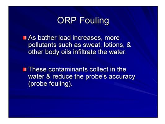
As the bather load increases, more pollutants like sweat, lotions and other body oils can infiltrate the water. These contaminants will collect in the water and reduce the probe's accuracy, known as probe fouling.
