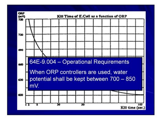
In the background is a chart that shows how many seconds it takes to kill E.coli according to how high the ORP controller is set. The higher the millivolts are the quicker the kill time will be. Under the state code for public pools, ORP controllers shall be kept between 700 and 850 millivolts.
