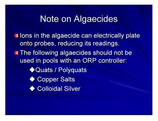
A note on algaecides, the ions in algaecides can electrically plate onto the probes, reducing their readings and effectiveness. You should not use these algaecides on any pools with ORP controllers: quats and polyquats, copper salts and colloidal silver.
