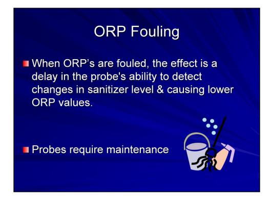
When ORPs are fouled, they can delay the probe's ability to detect changes in the sanitizer level and can cause lower ORP values. Your ORPs require regular maintenance.
