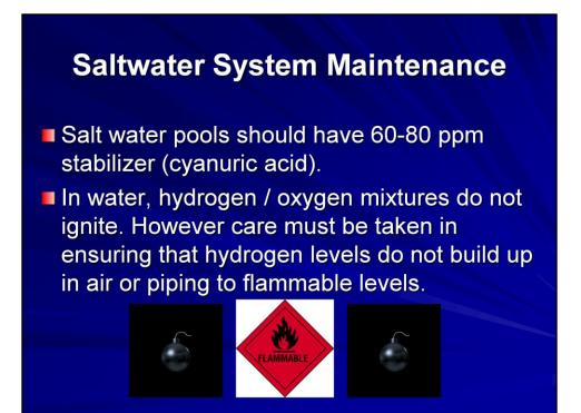
Salt water pools should have around 60-80ppm of cyanuric acid to maintain proper levels. In water, hydrogen/oxygen mixtures don't ignite. However, care must be taken in ensuring that hydrogen levels do not build up to flammable levels in the surrounding air or in the piping.
