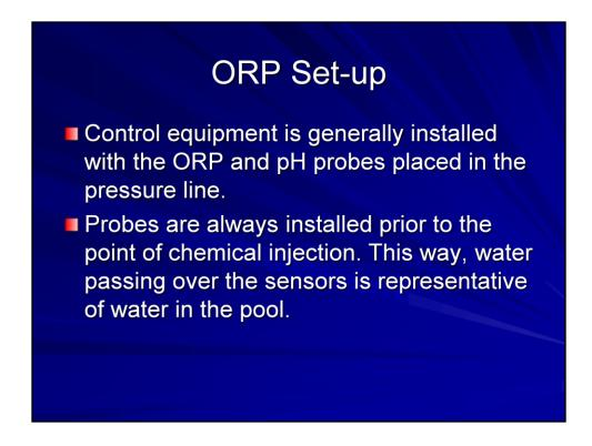
The control equipment is generally installed with the ORP and pH probes placed in the pressure line. The probes are always installed prior to the point of chemical injection. This way the water passing over the sensors is similar to the water in the pool.
