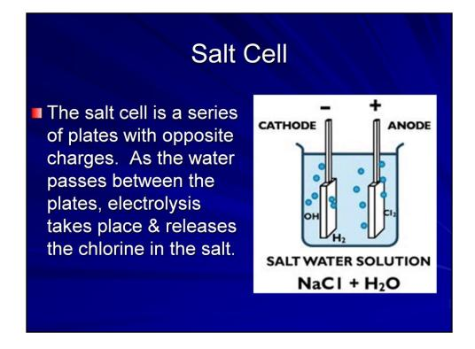
This is an example of the salt cell. The plates are oppositely charged, and as water passed between the plates, electrolysis takes place and releases the chlorine in the salt.
