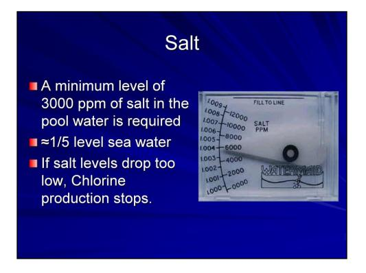
As I said before, a minimum of 3,000ppm of salt is required to maintain the system properly with adequate chlorine. This amount is equal to 1/5 the level of salt in sea water. Remember, if your salt levels drop too low, the production of chlorine will stop.
