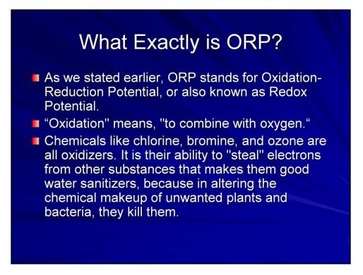
As we stated earlier, ORP stands for oxidation reduction potential, or redox potential. Oxidation means "to combine with oxygen." Chemicals like chlorine, bromine and ozone are all oxidizers. It is their ability to steal electrons from other substances that makes them good water sanitizers, because in altering the chemical makeup of unwanted plants and bacteria they kill them.
