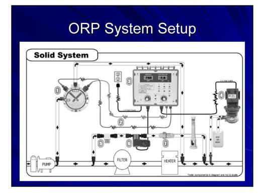
. This diagram shows an ORP system set up on a solid system, or an erosion system.
