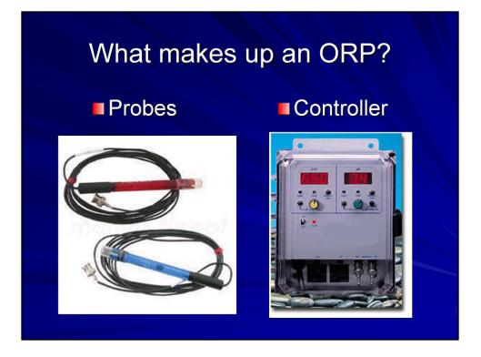
An ORP is made up of probes and a controller. The probes indicate the oxidizing/reducing capability of pool water by measuring the electron activity. The ORP probe reading signals the controller to adjust the chemical feeds as needed.
