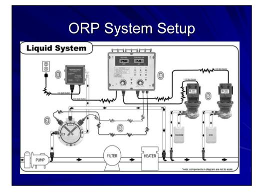
This is a diagram of an ORP system set up with liquid chemicals. Water goes into the cylinder with the probes to be read and sent to the controller, which will adjust the liquid chemicals as necessary.
