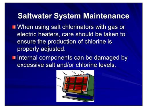
When using salt chlorinators with gas or electric heaters, care should be taken to ensure the production of chlorine is properly adjusted. Internal heater components can be damaged by excessive levels or chlorine and/or salt.
