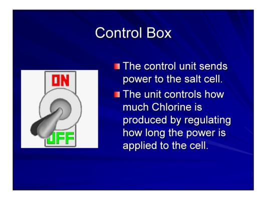
. The control box is the unit that sends power to the salt cell. The unit can control how much chlorine is produced by regulating how long the power is applied to the cell. The control box will also reverse the charges of the plates to prevent scale buildup on them.
