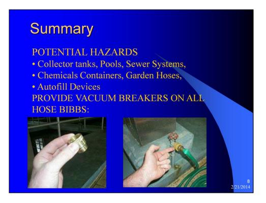
Cross connection hazards can be from collector tanks, pools, sewer systems, chemical containers, hoses and autofill devices. All hose bibs should have vacuum breaker devices installed.
