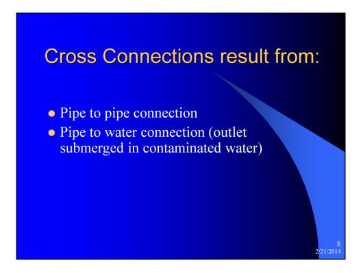
Cross connections can result from pipe to pipe connection, or from pipe to water connection, where the water outlet is submerged in contaminated water...like leaving a hose in dirty water.
